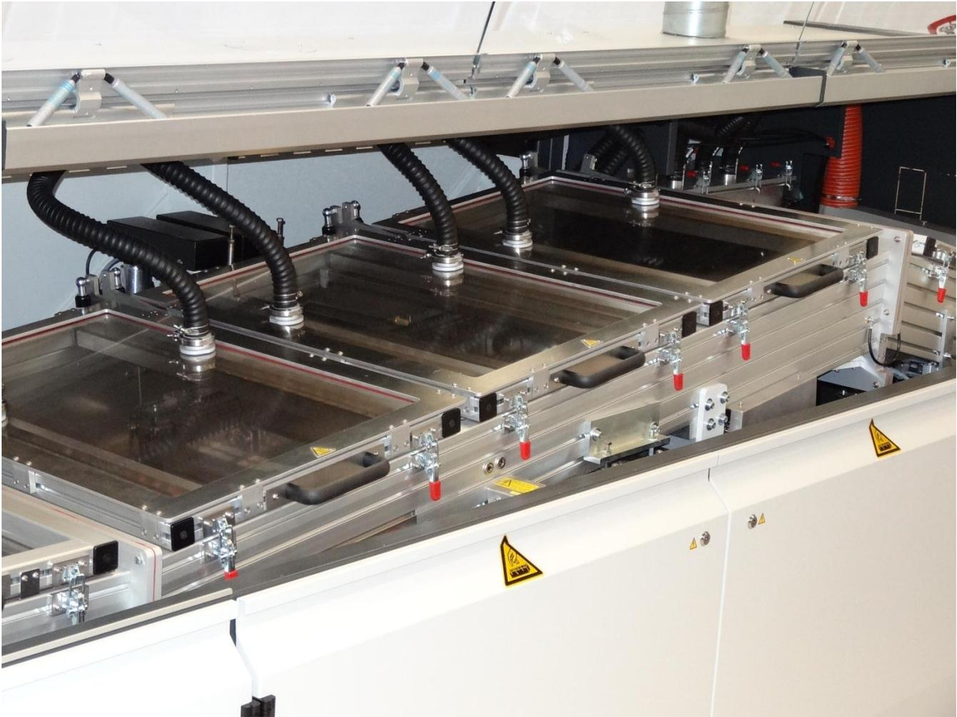
Fig 1. Sealed nitrogen tunnel to ensure stable and low residual oxygen levels
